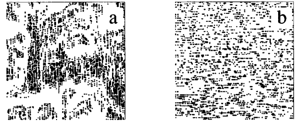
FIG. 7. Peak-peak distributions of the surfaces prepared at temperatures of -50\text{ }^\circ\text{C} (a) and 120\text{ }^\circ\text{C} (b).
